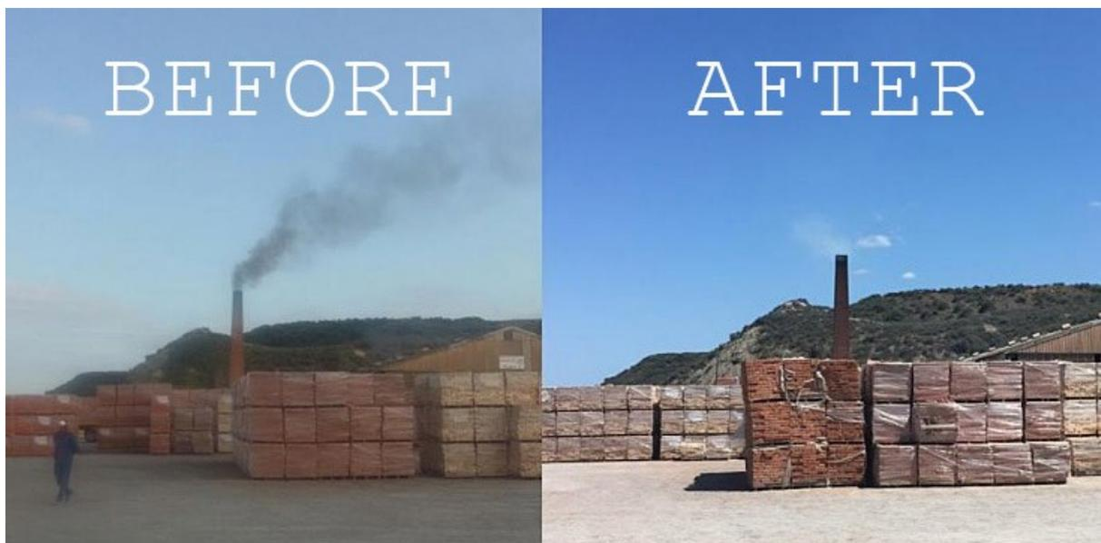
The post-implementation period recorded a 12.0% increase in the quantity of bricks packaged for sale. A portion of this came from an increased throughput of 4.6% but much can be attributed to the waste reduction of 6.1%. This waste reduction can be attributed to more even and effective burning of the fuel which serves to optimise the energy obtained from the fuel and minimise any negative effects such as flame impingement.
