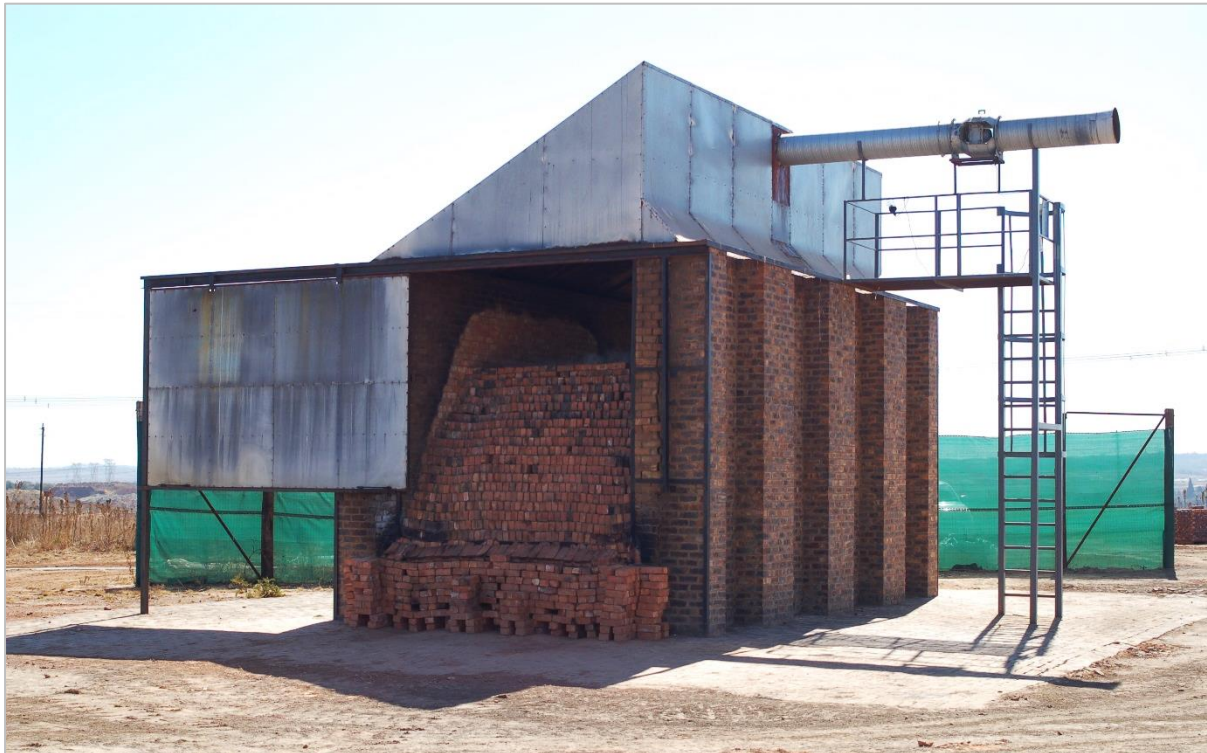
Figure 2: Model Kiln with horizontal stack and mesh windscreen Source: Akinshipe and Kornelius (2007)
